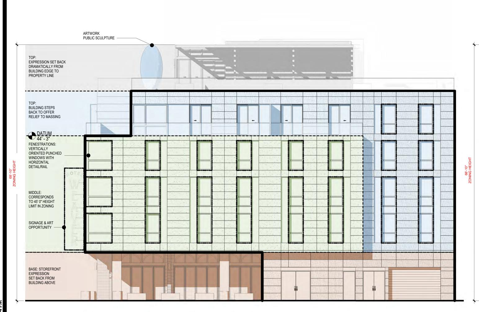
VERTICAL MOVES: BALCONY RECESSES AND NOTCH READS VERTICALLY TO BREAK UP MIDDLE, HORIZONTAL MASSING ARTWORK PUBLIC SCULPTURE EXPRESSION SET BACK DRAMATICALLY FROM **BUILDING EDGE TO** -----BUILDING STEPS BACK TO OFFER RELIEF TO MASSING FENESTRATIONS: VERTICALLY ORIENTED PUNCHED WINDOWS WITH HORIZONTAL DETAIL/RAIL CORRESPONDS TO 45' 0" HEIGHT LIMIT BASE: STOREFRONT EXPRESSION SET BACK FROM BUILDING ABOVE SIGNATE & ART OPPORTUNITY — 26' - 3 1/2" 24' - 11" 13' - 5" 25' - 11"
